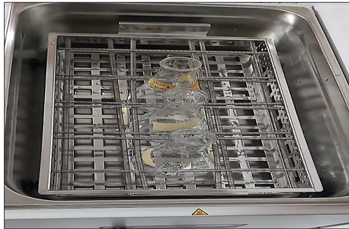
Figure 2. Shaking device with water path
