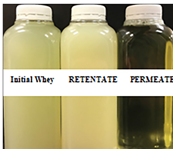
Figure 3. Initial whey, permeate, and retentate after diafiltration
