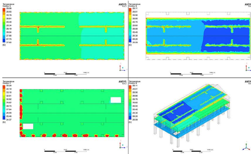
Figure 12. Temperature distribution on the horizontal section of traditional Rumoh Aceh (XZ plane) at 12:00 WIB
