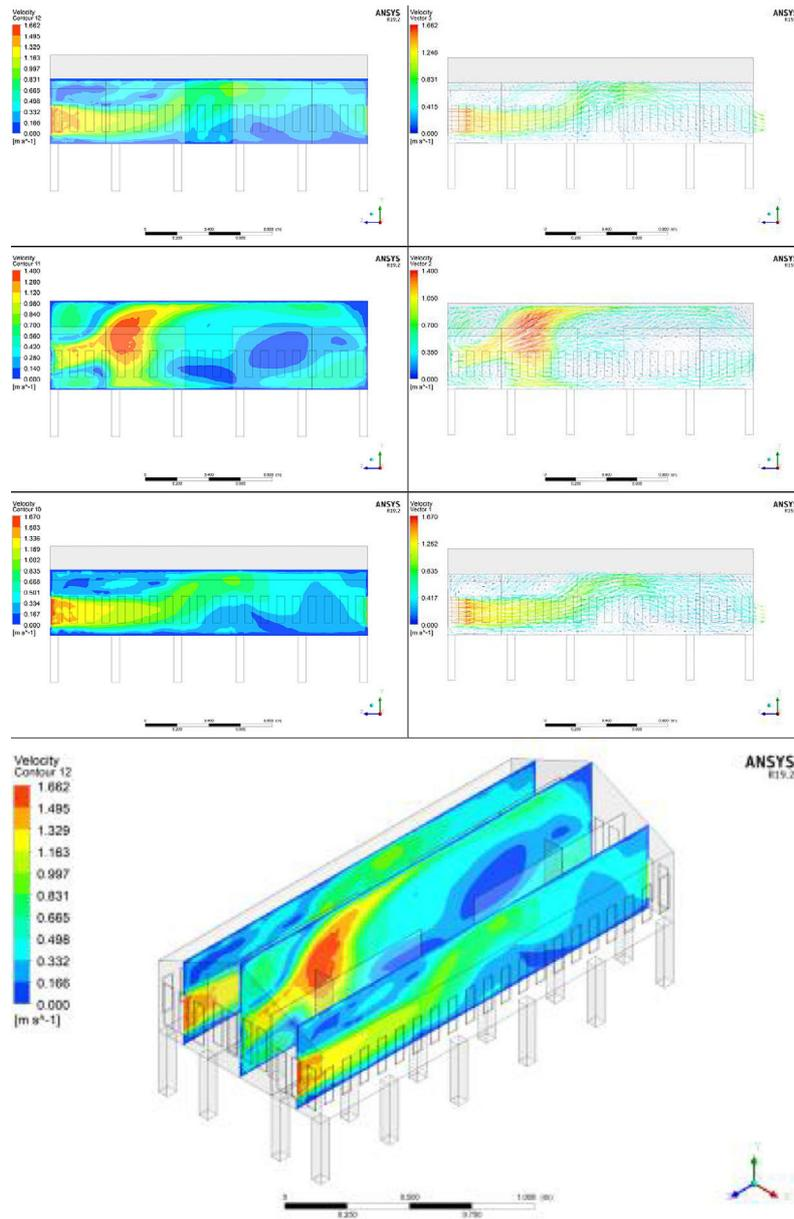
**Figure 7.** Velocity distribution on the longitudinal vertical section of traditional Rumoh Aceh (YZ plane)
