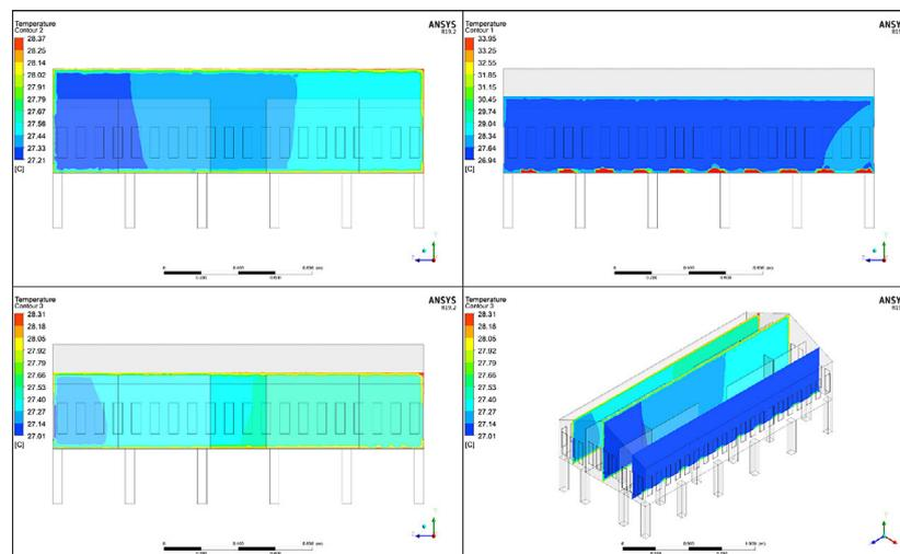
Figure 16. Temperature distribution on the longitudinal vertical section of traditional Rumoh Aceh (YZ plane) at 16:00 WIB
