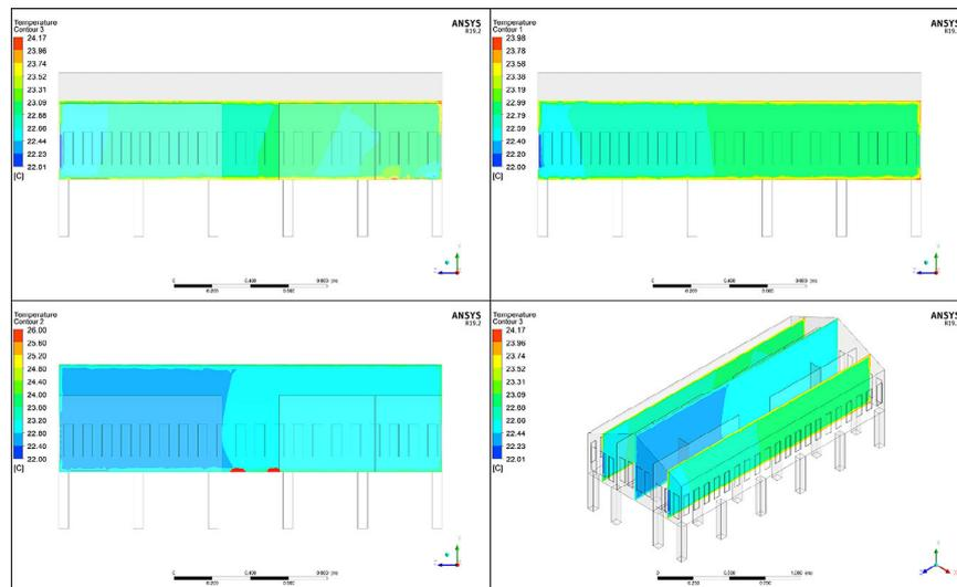
Figure 10. Temperature distribution on the longitudinal vertical section of traditional Rumoh Aceh (YZ Plane) at 08:00 WIB
