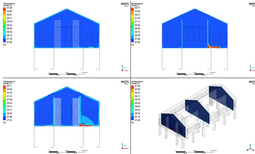
Figure 14. Temperature distribution on the vertical section of traditional Rumoh Aceh (XY plane) at 16:00 WIB
