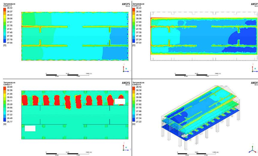
Figure 15. Temperature distribution on the horizontal section of traditional Rumoh Aceh (XZ plane) at 16:00 WIB
