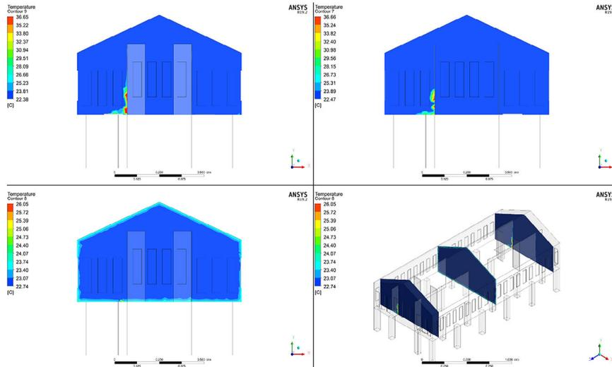
Figure 8. Temperature distribution on the vertical section of traditional Rumoh Aceh (XY plane) at 08:00 WIB
