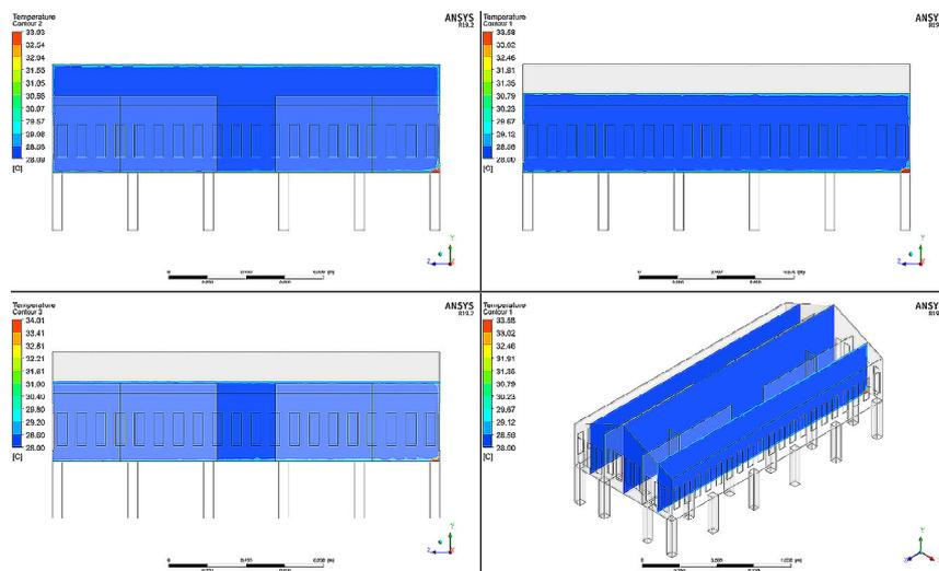
Figure 13. Temperature distribution on the longitudinal vertical section of traditional Rumoh Aceh (YZ plane) at 12:00 WIB
