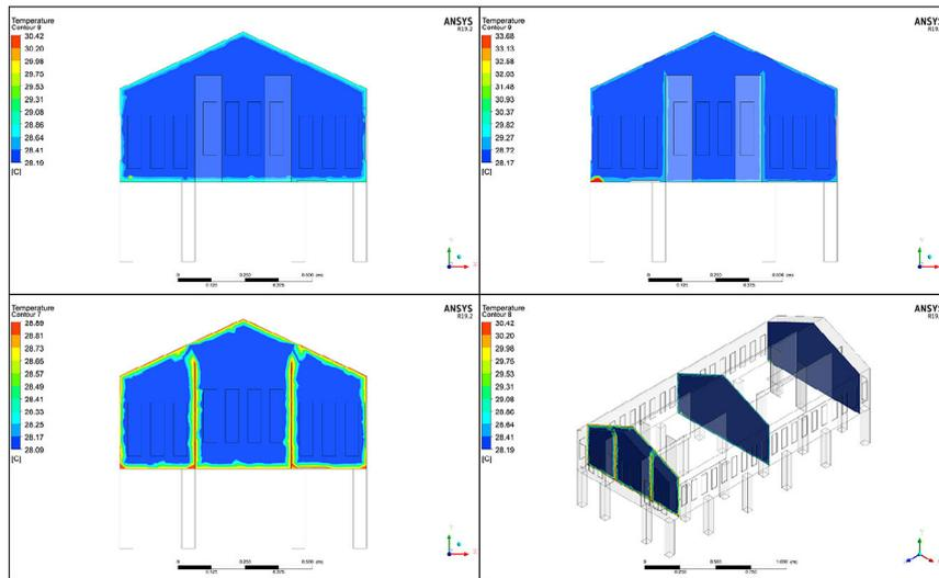
Figure 11. Temperature distribution on the vertical section of traditional Rumoh Aceh (XY plane) at 12:00 WIB
