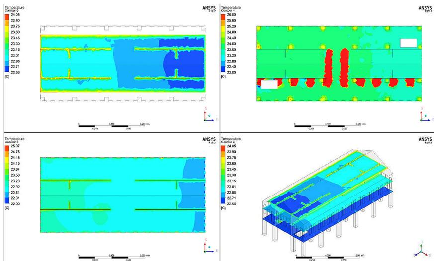
Figure 9. Temperature distribution on the horizontal section of traditional Rumoh Aceh (XZ plane) at 08:00 WIB
