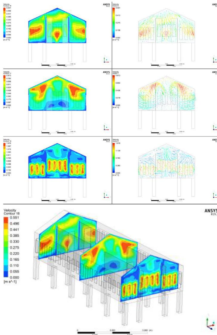
Figure 5. Velocity distribution on the vertical section of traditional Rumoh Aceh (XY plane)
