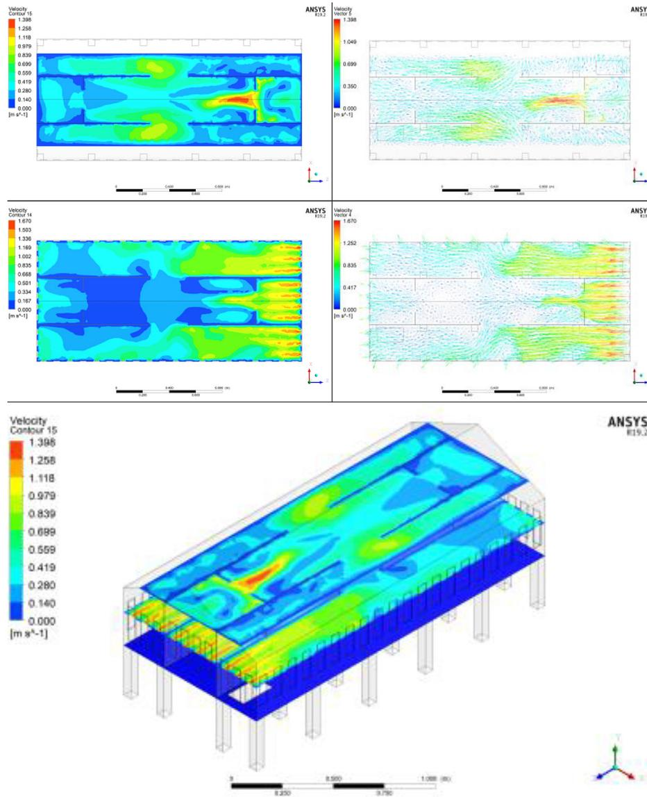
Figure 6. Velocity distribution on the horizontal section of traditional Rumoh Aceh (XZ plane)
