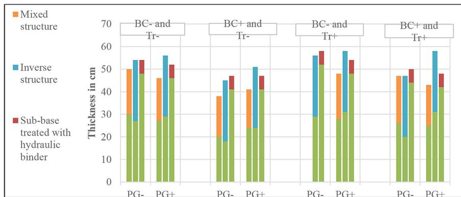
Figure 14. Effect of each factor on PG layer thickness and total pavement thickness
