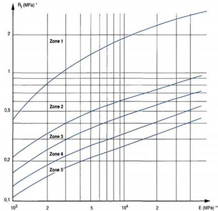
Figure 1. Classification chart of treated materials for subgrade layer
