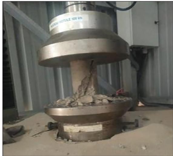
**Figure 5.** Simple compressive strength (NF EN 13286-41)
