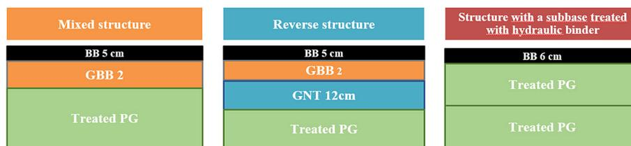
Figure 10. Types of pavement structures considered in the parametric study (Diouri et al., 2022)
