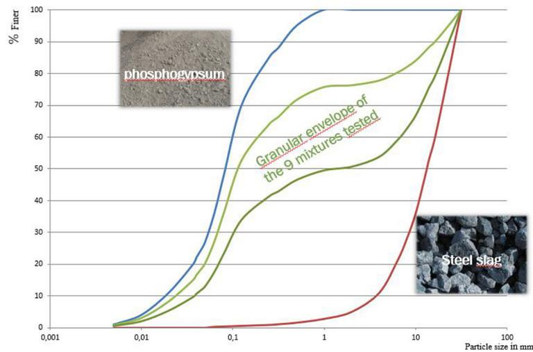
Figure 8. Particle size distribution of PG, SS, and the 9 mixtures of the PG-SS-C formulation
