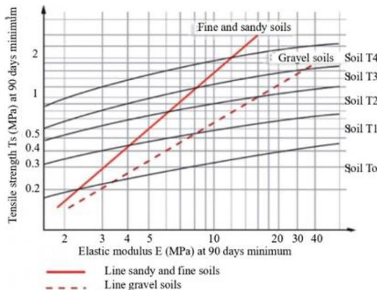
Figure 2. Classification chart of treated materials for the foundation layer
