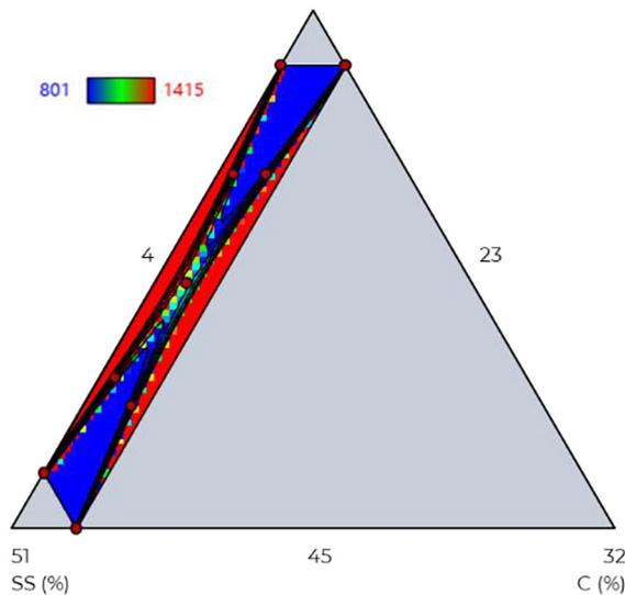
**Figure 11.** Elastic modulus E28d modeling for PG-SS-C mixtures
