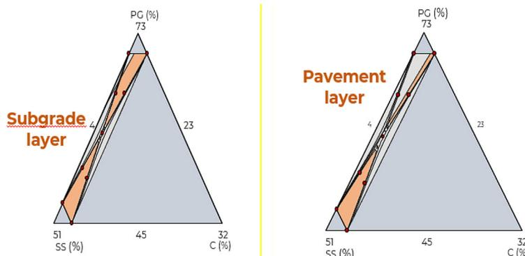
**Figure 13.** PG-SS-C: suitable domain either for subgrade or foundation layer
