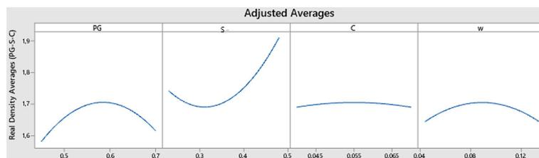
**Figure 12.** Main effects diagram, Proctor modeling
