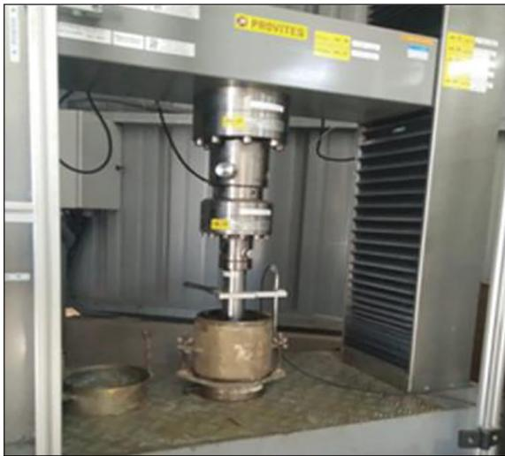
**Figure 3.** Immediate bearing index (NF P 94-078)
