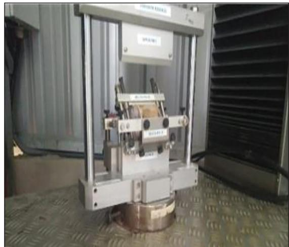
**Figure 6.** Diametral tensile strength and elastic modulus (NF P 98-232-3)
