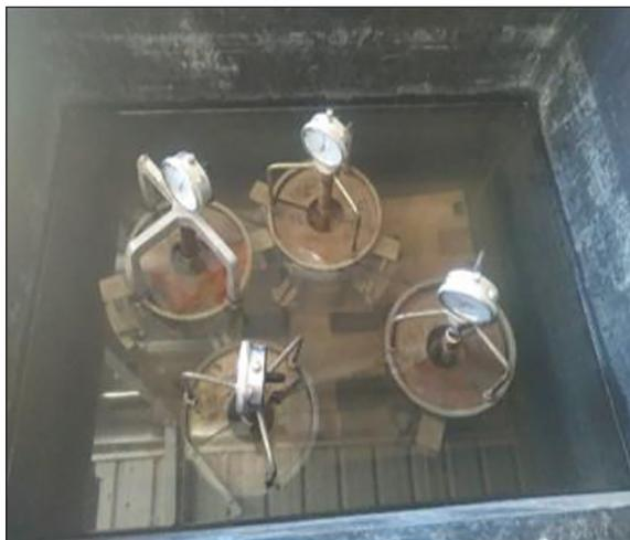
**Figure 4.** Californian bearing ratio after 4 days of water immersion and vertical swelling after 4 days of water immersion with overload (NF P 94-078)
