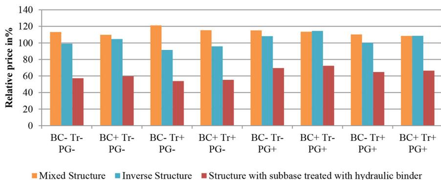
Figure 15. Relative price estimation of the mixed/inverse/treated pavement structure compared to a conventional structure (thick bituminous)
