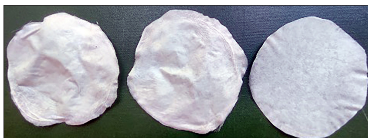
Figure 4. Visual appearance of cellulose membrane samples obtained by different drying methods (from left to right): in the drying part of the laboratory hand sheet forming equipment (120 °C), on the drying cylinder (90 °C), at ambient air temperature (28 °C)
